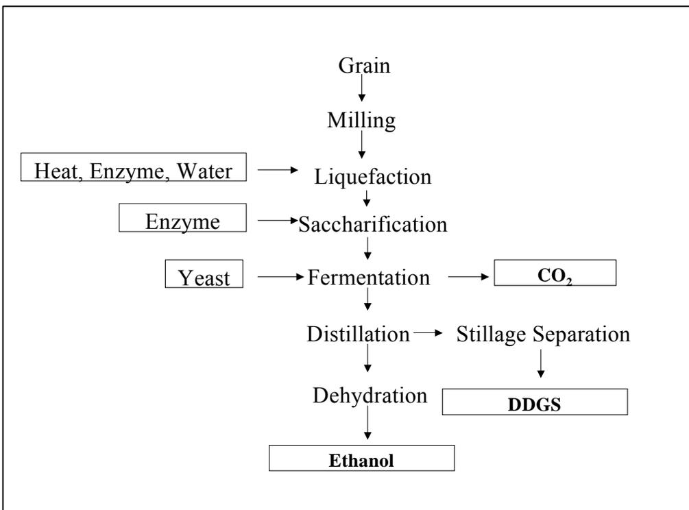
**Figure 1 - Overview of the basic “dry grind” process of fuel alcohol production.** The products ethanol, DDGS and CO<sub>2</sub> are produced in approximately equal amounts by weight.
