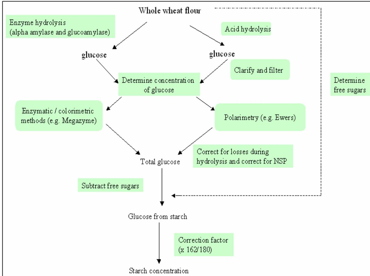
**Figure 7 - Overview of the enzymatic and acid hydrolysis methods of quantifying starch.**
